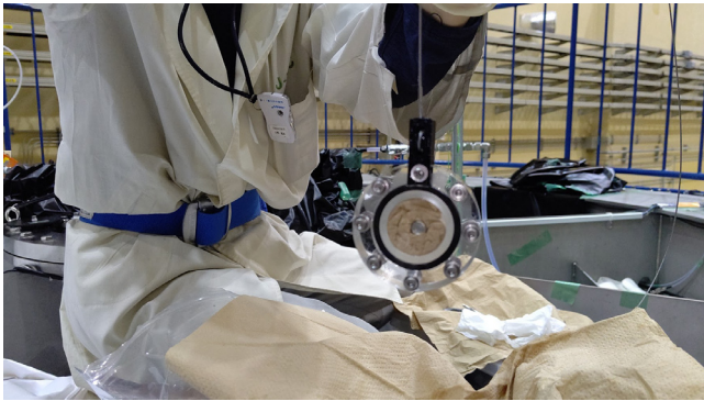
Fig. 28. The JSNS 2 252 Cf calibration source inside an acrylic container.
