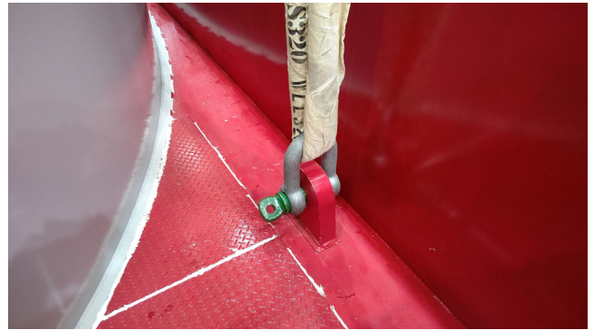
Fig. 6. A shackle tied to the detector. Four shackles are used to lift the detector.
