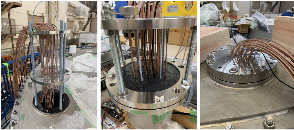
Fig. 13. PMT cable flanges. Left: A flange consists of double layers. Center: The lower layer is filled with the epoxy resin. Right: The top layer is used to close the flange.
