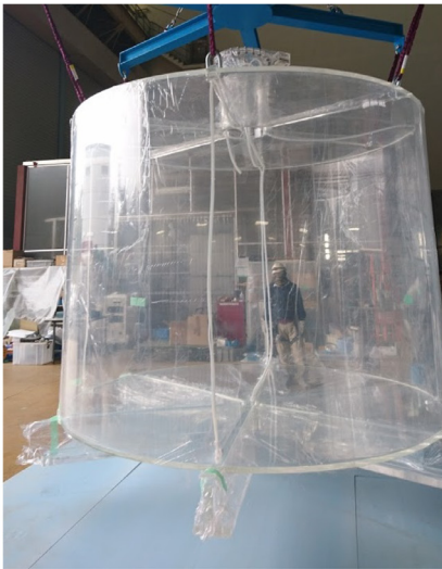
Fig. 7. Schematic drawing (top) and picture (bottom) of the acrylic vessel. The dimensions are given in mm.
